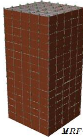
Fig.5: 15 story, 5 bay MRF views, with and without infills (regular)
